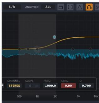
The filter band listen mode enables the listening of the output signal in a specific filter band with all DSEQ processing. Filter frequency and Q are determined by the selected pre-filter. Just click on one of the pre-filter buttons (no need to be active) and move button around.
